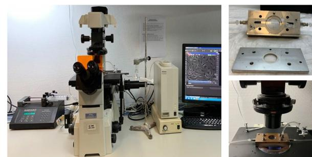
**Figure 2. Microscope and parallel-plate flow chamber.**
